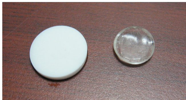
Fig. 1. Appearance of gel F-50 in the water-swollen state (left) and the dry, extracted state (right).
